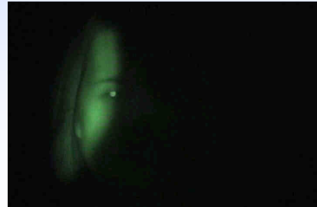
Using telescope + NIR illuminator (30 m)
