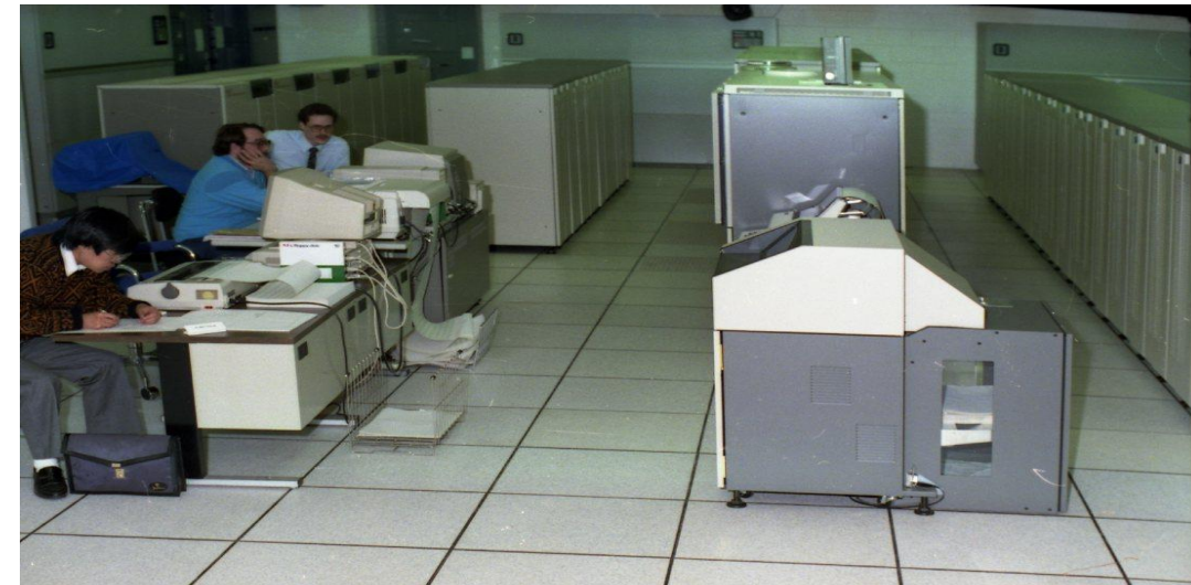
MSP AFIS (1989): 700K tenprints in database; 5K rolled print searches; no latent search; 15K comparisons/sec.
