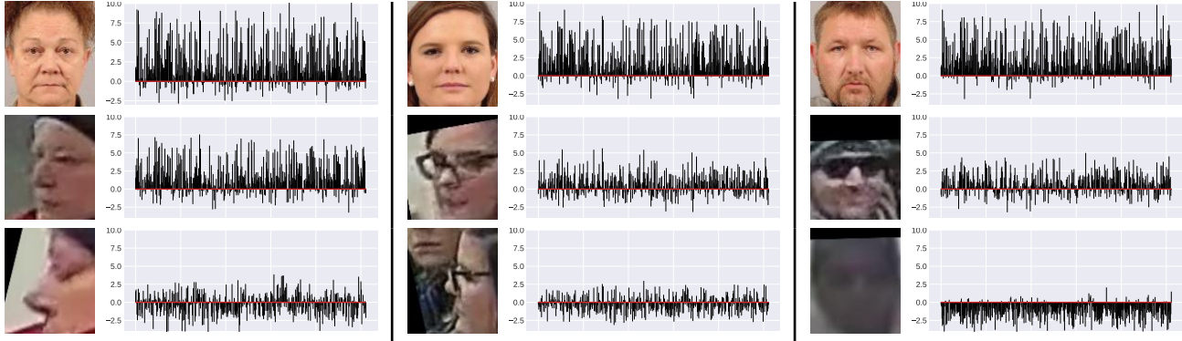
Figure 5: Component-wise quality scores given by C-FAN for images of three subjects in the IJB-S dataset. Unnormalized quality scores are shown here for fair comparison. In the plots, quality values are shown for each of the 512 components. Each column shows a high-quality photo, a medium-quality frame and a low-quality frame from the same person, respectively.
