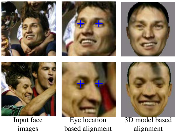
Fig. 6. Alignment results of two unconstrained face images of one subject from the LFW+ database by (i) 2D affine transformation (based on eye locations) and (ii) 3D face model (A COTS 3D modeling system, CyberExtruder Aureus 3D SDK 11 , is used in our approach).
