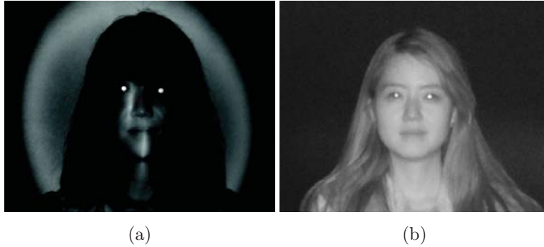
Figure 2: Nighttime NIR images at 60m standoff: (a) the NIR illuminator used in [11] introduces halo like light pattern around the head; (b) an improved NIR illuminator used in this paper leads to much better image quality compared to (a).
