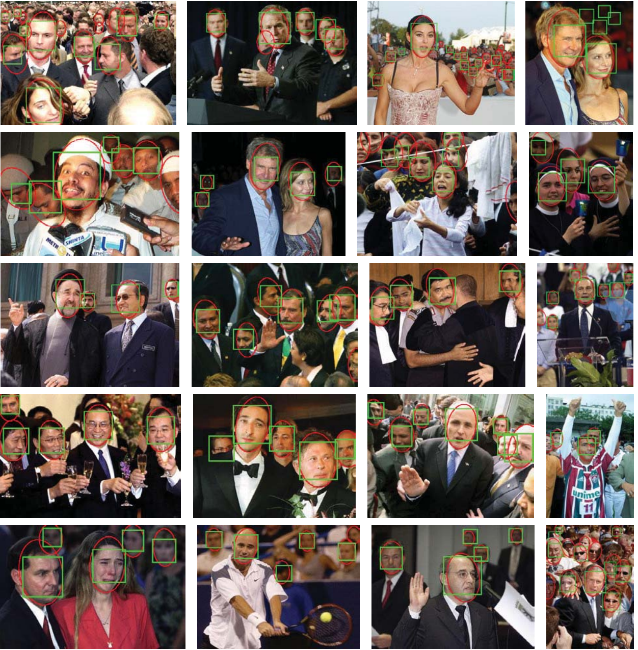
Fig. 10. Detected faces in the Fddb database [3] by the proposed NPD method. Green boxes are detections by the proposed method, while red ellipses are ground truth annotations.
