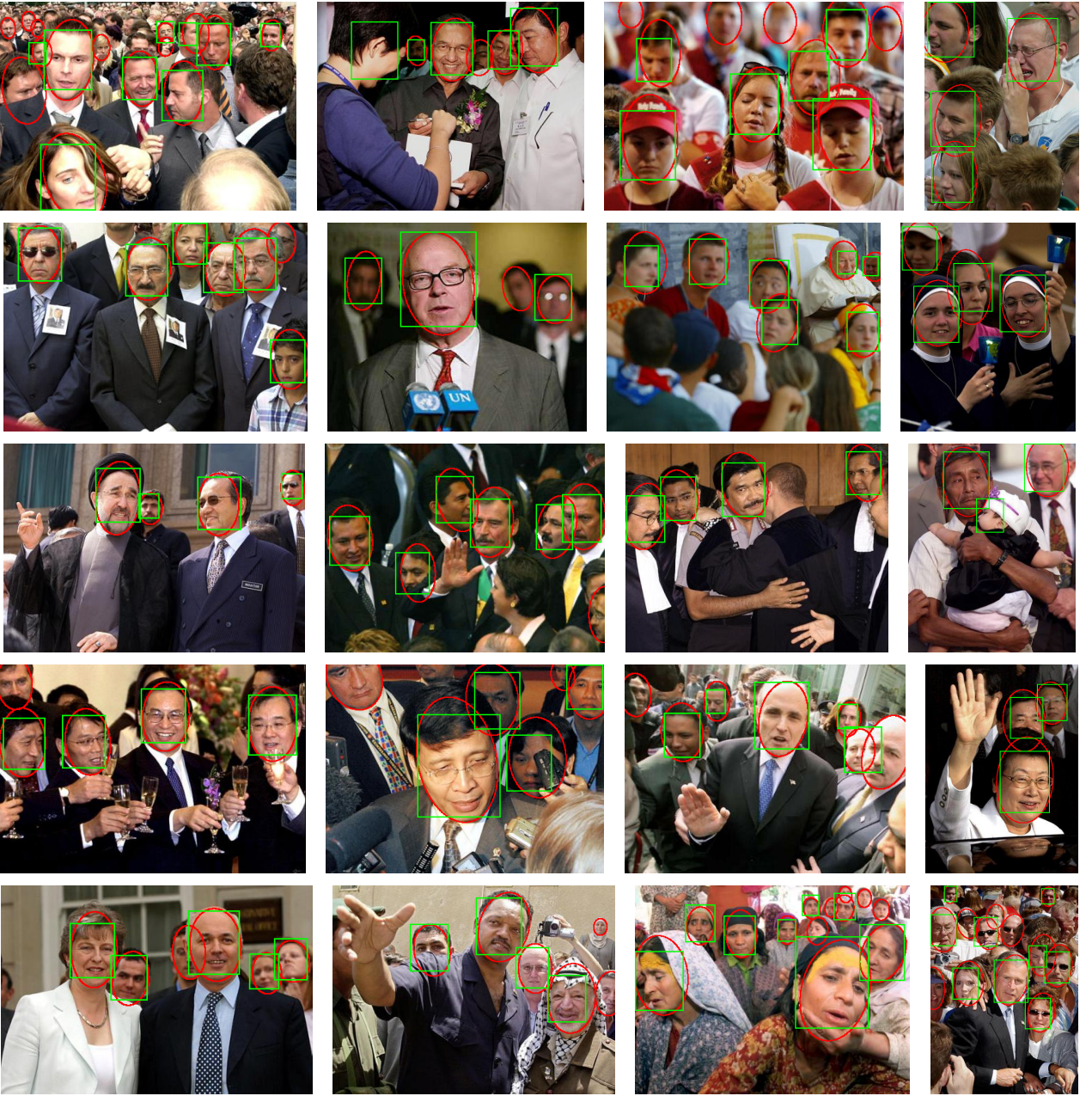
Fig. 7. Detected faces in the Fddb database [3] by the proposed NPD method. Green boxes are detections by the NPD detector, while red ellipses are ground truth annotations.
