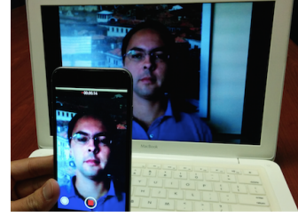
Figure 3. Demonstration of how replay attack videos are collected, using a laptop screen as the spoof medium and a smartphone as an acquisition device. This simulates how a user may launch an attack against a FR system by using a video/image found online.
