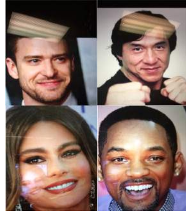
Fig. 7. Examples of spoof attacks launched using a digital screen show evidence of surface reflection. The top row shows bright indoor lighting reflecting off a digital screen. The bottom row shows the screen of a mobile device reflecting the image it's capturing.
