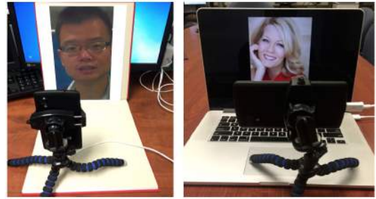
Fig. 6. Demonstration of how samples of (a) print attacks, and (b) display and replay attacks were collected, using paper and laptop screen as the spoof medium and a smartphone as an acquisition device. This simulates how a user may launch an attack against a FR system.
