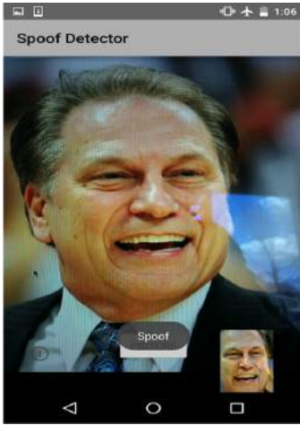
Fig. 20. The GUI of our android application. The figure shows the recaptured image of a face replay attack on a MacBook Pro screen; as shown on the Nexus 5 screen, the application successfully detected the input as a spoof access. The face image in the bottom-right corner displays the detected face.
