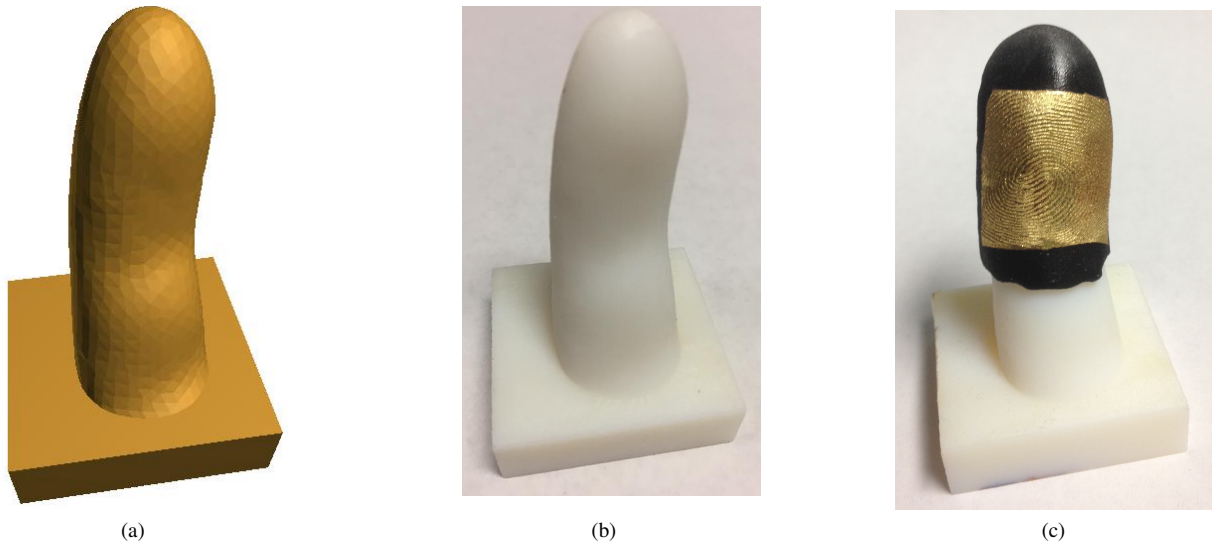
Fig. 6. 3D mount fabricated (using Stratasys Objet Connex350) to hold a 3D target for stable placement on the sputtering system's rotary platform. (a) Electronic 3D model, (b) 3D printed physical model and (c) 3D fingerprint target on the mount shown in (b) after gold coating.
