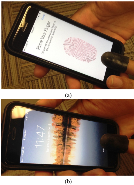
Fig. 12. Evaluation of capacitive readers embedded in smartphones using gold fingers. (a) Enrollment of a gold finger on an Apple iPhone 6s, and (b) unlocking of the iPhone 6s using the same gold finger.
