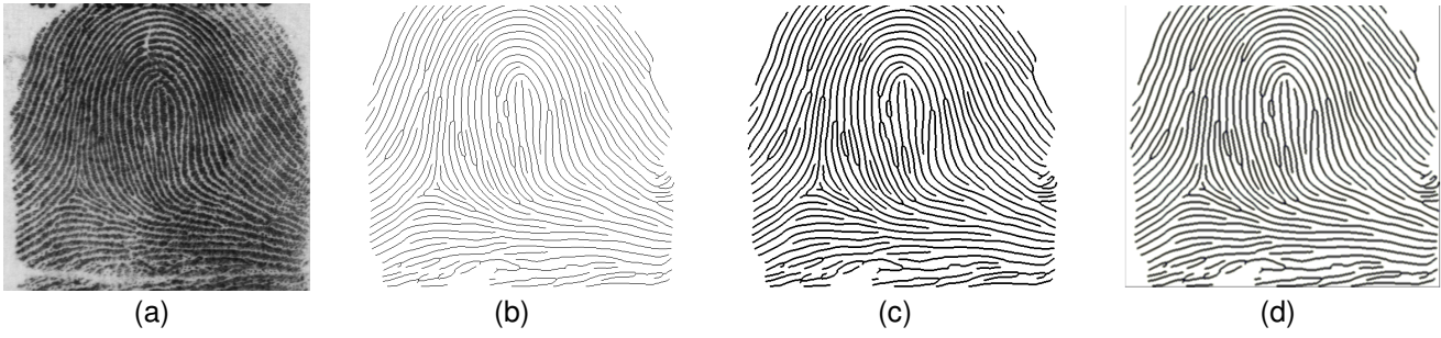
Fig. 5. Preprocessing a 2D fingerprint pattern before projection onto 3D finger surface. (a) Original fingerprint image, (b) extracted skeleton of the fingerprint in (a), (c) skeleton in (b) after applying the morphological operation of dilation, and (d) dilated skeleton in (c) smoothed using a gaussian filter.
