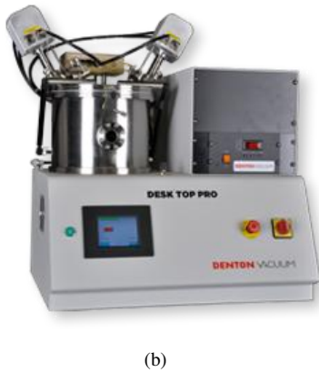
Fig. 4. DC sputter deposition to coat the 3D targets, fabricated using a high-resolution commercial 3D printer, with thin layers of conductive materials. (a) Simplified representation of the DC sputtering process (image reproduced from [19]), and (b) the Denton Vacuum DC sputtering system [20] used for DC sputtering. Conductive material from the cathode target (titanium (Ti) and gold (Au) used here) is deposited on the anode substrate (3D target) using Argon (Ar) as the process gas.
