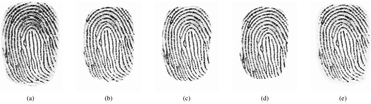
Fig. 11. Five different impressions of a gold finger captured using the large area PIV certified capacitive reader. The center-to-center ridge spacing measurements in each impression are used for the evaluation of the reader.
