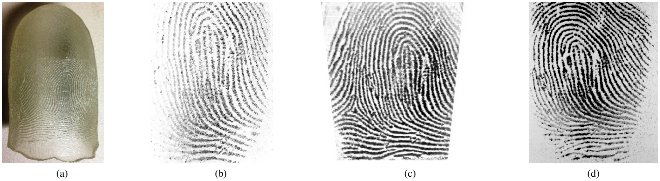
Fig. 2. Images of a 3D fingerprint target fabricated with translucent rubber-like material TangoPlus FLX930 [5] (shown in (a)) captured by three different PIV certified [1] single-finger optical readers using different wavelengths of light for fingerprint capture: (b) blue wavelength, (c) combination of blue and red wavelengths, and (d) red wavelength. Targets printed with black colored rubber-like materials (TangoBlackPlus FLX980 [5] and FLX9840-DM [9]) could not be imaged using these three readers.
