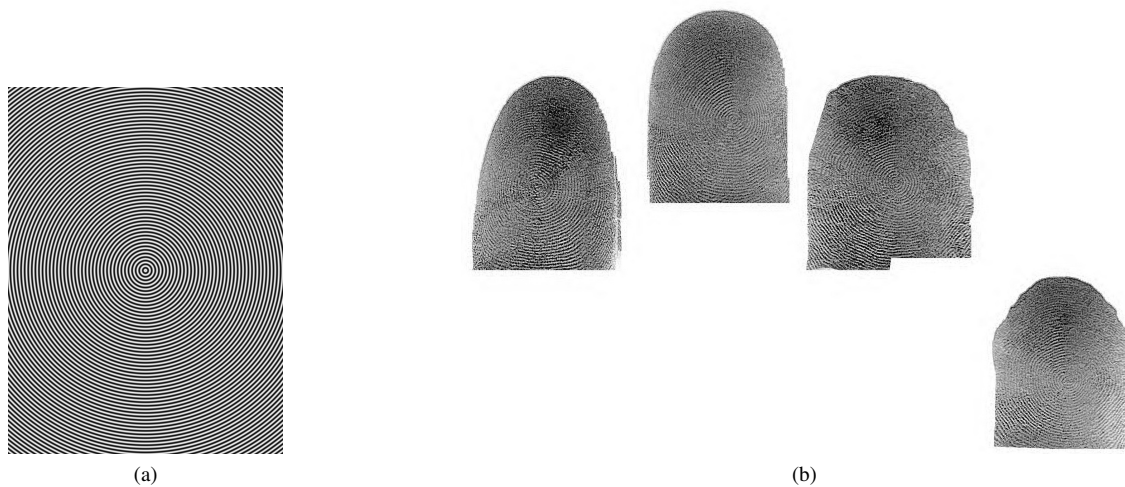
Fig. 5. Circular sine grating (ridge spacing = 10 pixels) used to generate the 3D whole hand target (shown in (a)) and the slap impression of the corresponding hand target captured using the contactless slap reader (shown in (b)).
