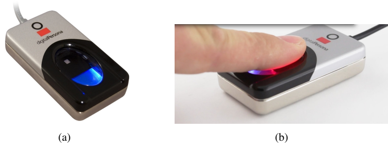
Figure 5: (a) The 500 ppi Digital Persona U.are.U 4500 HD fingerprint reader [18] used to collect child fingerprints. The approximate reader size is 65 mm x 36 mm x 15.56 mm and it weighs 105 grams. (b) A red light glows once the finger is placed on the reader platen to trigger the fingerprint image capture.
