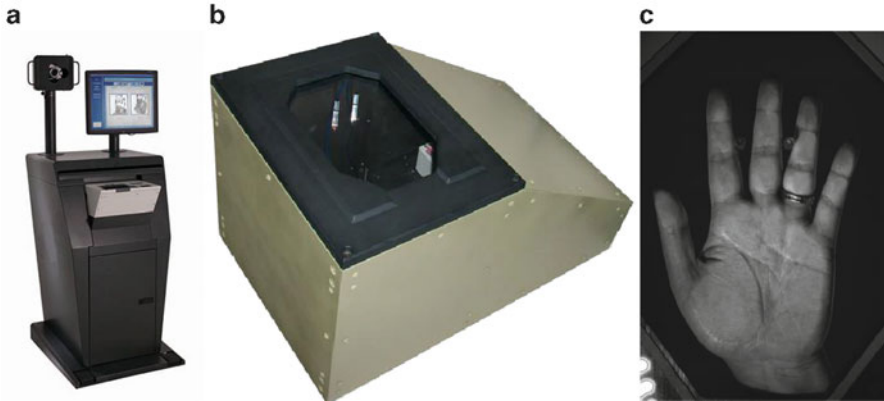
Fig. 3.9 Multibiometric data acquisition. (a) A multibiometrics acquisition system from Printrak (Printrak Division) to acquire fingerprints, palmprints, face images, iris images, signature details and soft biometrics data such as scars and tattoos; (b) full hand multispectral scanner from Lumidigm (Rowe et al. 2007) and (c) a sensed hand image from (b)
