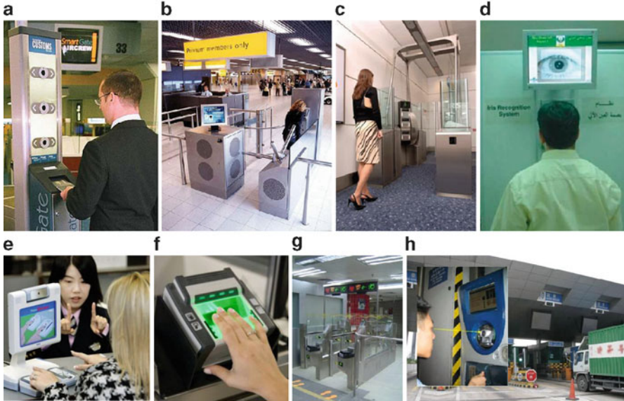
Fig. 3.2 Deployment of biometrics systems at border crossings for immigration control; (a) face recognition system (SmartGate) at Sydney airport (Australian Government), (b) iris recognition system at Amsterdam Schiphol airport (Schiphol), (c) at Manchester airport (UK) (Ranger 2006) and (d) at UAE airport (Daugman and Malhas 2004); (e) fingerprint recognition using index fingers at airports in Japan (Higaki 2007); (f) ten fingerprint acquisition at airports in the United States (US Department of Homeland Security); (g) fingerprint based immigration clearance for passengers at Hong Kong airport; (h) vehicular clearance using fingerprint and face in Hong Kong (E-Channel)
