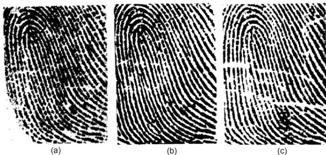
Fig. 18. Herschel’s fingerprints at age 7 (a), age 17 (b), and age 40 (c). The pairwise match scores of a state-of-the-art fingerprint matcher for these three fingerprints are: (a) vs. (b) 6,217; (a) vs. (c) 5,032; (b) vs. (c) 5,997; the maximum impostor score of (a) against 10,000 fingerprints in NIST SD4 is 3,325 and that of (b) is 2,935, implying that these three fingerprint images can be claimed to originate from the same finger with high confidence.
