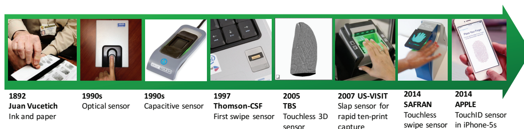
Fig. 9. Evolution of fingerprint sensing technology. Fingerprint sensors have evolved in two ways. On the one hand, they have become compact in size and cheaper in cost, which makes it possible to embed fingerprint sensors in devices such as laptops or mobile phones. While some applications still use a large surface area fingerprint sensor (for capturing a full fingerprint impression resulting in higher accuracy), they are equipped with several advanced functionalities. A typical example is the slap sensor used in the US-VISIT program (Department of Homeland Security, 2013), which can capture impressions of multiple fingers simultaneously, thereby facilitating rapid capture of ten-prints. Other examples include the 3D fingerprint sensor introduced by TBS in 2005 (Parziale and Diaz-Santana, 2006) and the touchless fingerprint sensor introduced by Safran in 2010 (Fourre et al., 2011), which can acquire the images of multiple fingers on-the-fly as the user moves his hand across the device.
