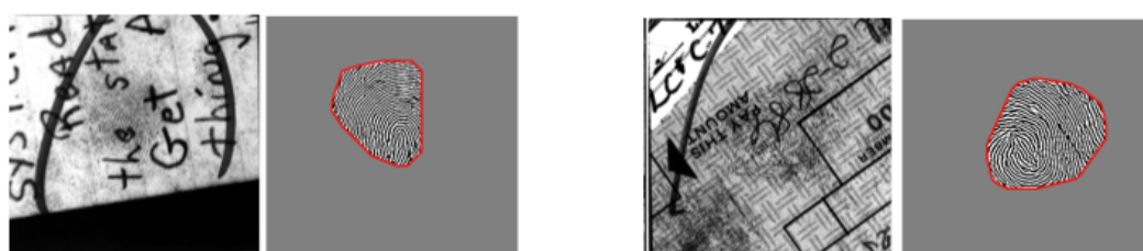
Figure 9. Examples of two fingerprints that have been automatically enhanced using image processing techniques. Forensic experts can avail of the progress made in pattern recognition, computer vision, image processing and machine
