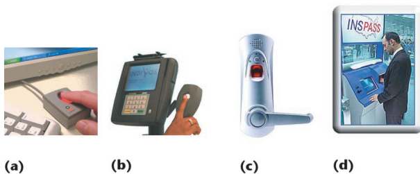
Figure 4. Biometrics application examples. (a) Digital Persona's fingerprint verification system provides personal recognition for computer and network login. (b) Indivios manufactures a fingerprint-based point-of-sale (POS) terminal that verifies customers before charging their credit cards. (c) BioThentica's fingerprint-based door lock restricts access to premises. (d) The Inspass immigration system, developed by Recognition Systems and installed at major airports in the US, uses hand geometry verification technology.
