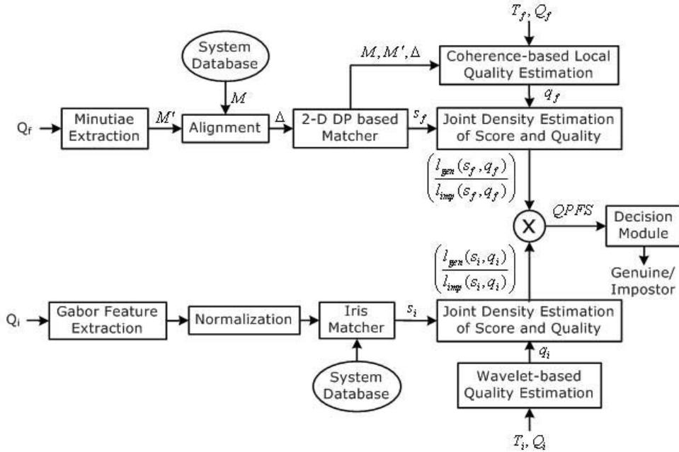
**Figure 1. Framework for quality-based fusion.** Here,  $T_f$  and  $Q_f$  ( $T_i$  and  $Q_i$ ) represent the template and query fingerprint (iris) images,  $s_f$  and  $q_f$  ( $s_i$  and  $q_i$ ) represent the fingerprint (iris) match score and quality,  $M$  ( $M'$ ) represents the template (query) fingerprint minutiae,  $\Delta$  represents the rigid transformation between  $T_f$  and  $Q_f$  and QPFS represents the quality-based product fusion score.
