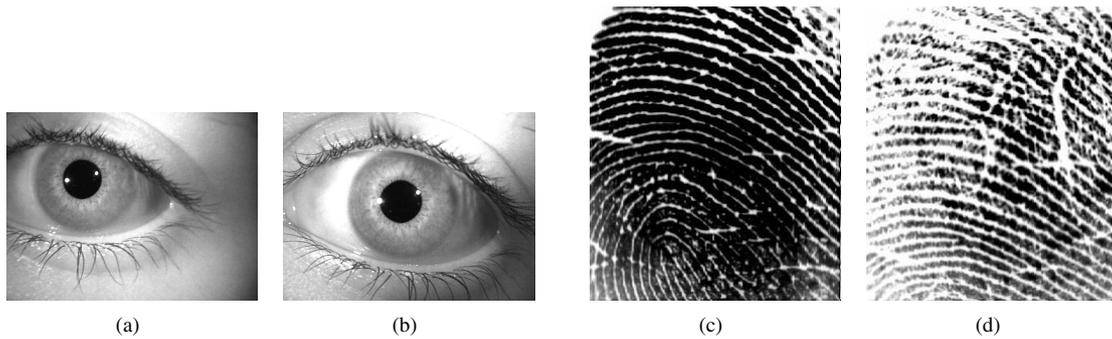
**Figure 3. Illustration of quality-based fusion. This user's iris images ((a) template and (b) query) are of good quality and the fingerprints ((c) template and (d) query) are of poor quality. Quality-based fusion rule implicitly assigns a higher weight to the iris modality, resulting in a correct acceptance of a genuine user who was falsely rejected by the simple product fusion rule.**
