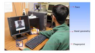
Figure 4: A prototype multimodal biometric login system.
