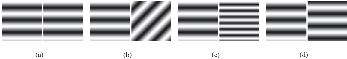
Fig. 6. Continuity of adjacent waves. (a) Two waves are continuous, (b) the direction of two waves is discontinuous, (c) the frequency of two waves is discontinuous, and (d) the normalized grayscale values of two waves are discontinuous.
