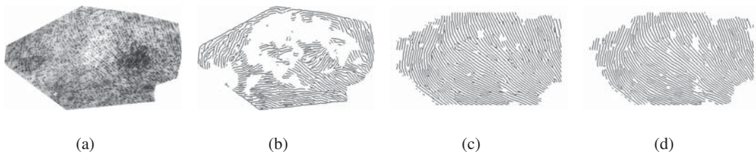
Fig. 9. Comparison of VeriFinger 6.0, the algorithm in [23] and the proposed algorithm for ridge detection. (a) A latent print (height: 523 pixels, width: 886 pixels), (b) skeleton image of (a) by VeriFinger, (c) skeleton image of (a) by the algorithm in [23], and (d) skeleton image of (a) by the proposed algorithm.
