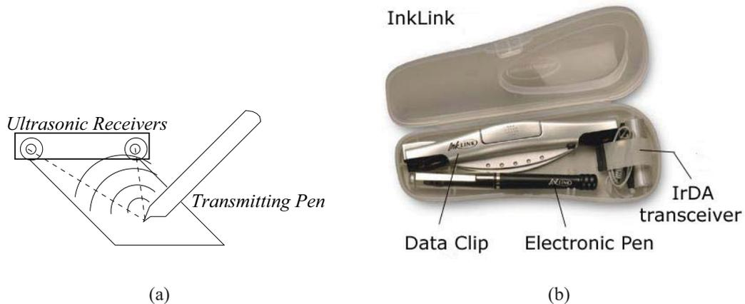
Figure 1.9: Ultrasonic Tracking: (a) schematic diagram of an ultrasonic position sensor and (b) the InkLink<sup>®</sup> sensor.
