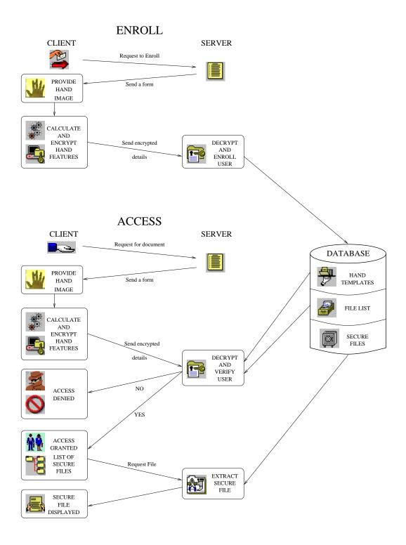
Figure 8: Flow diagram of client-server interaction.
