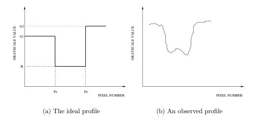
Figure 3: The gray scale profile of pixels along a measurement axis.
