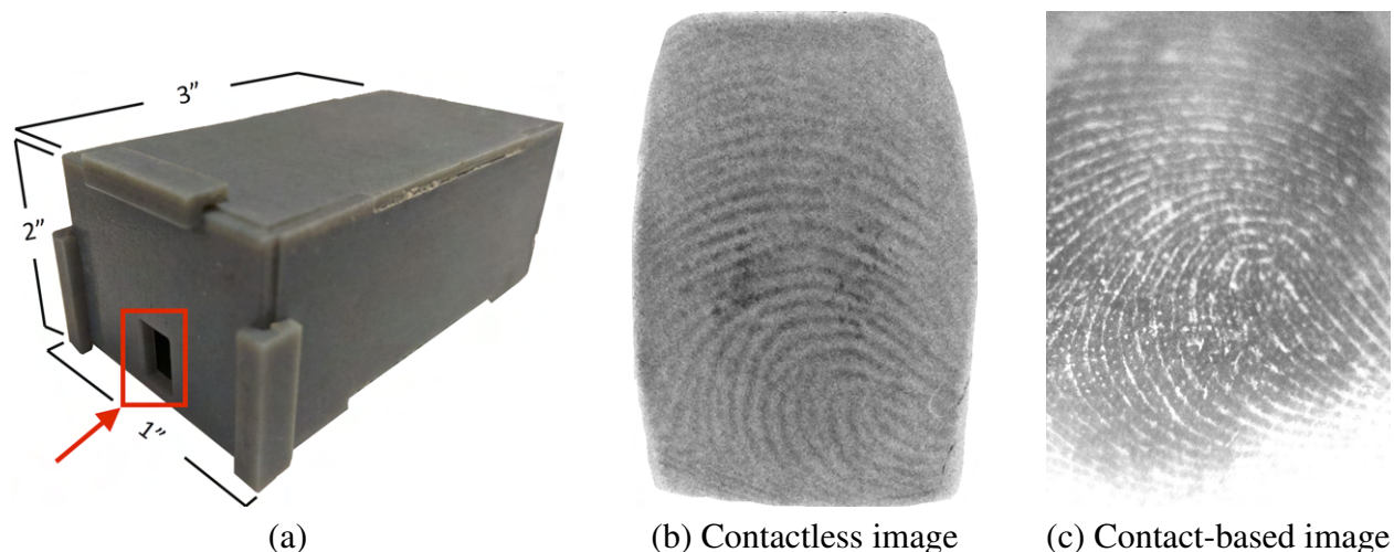
Figure 5.6 (a) Prototype of our 1,900 ppi contactless fingerprint reader. During capture, an infant’s finger is placed on top of a small, contactless, rectangular opening (annotated in red) on the reader (the size of this opening can be adjusted with different sized slots). A camera captures the infant’s fingerprint from behind the rectangular opening. Examples of a processed (segmented, contrast enhanced), contactless infant thumb-print (2 months old) is shown in (b) and the same infant’s thumb-print acquired via contact-based fingerprint reader in (c).
