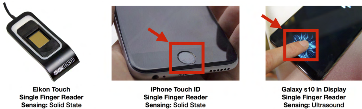
Figure 1.9 Examples of different types of solid-state readers (both capacitive) and an in-display, mobile-phone, ultrasound reader. Images retrieved from Google Images.
