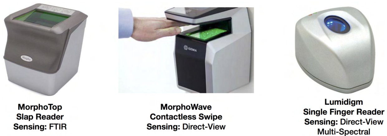
Figure 1.8 Examples of different types of optical-based fingerprint readers (Idemia https://www.idemia.com/ , HIDGlobal https://www.hidglobal.com/ ). Images retrieved from Google Images.
