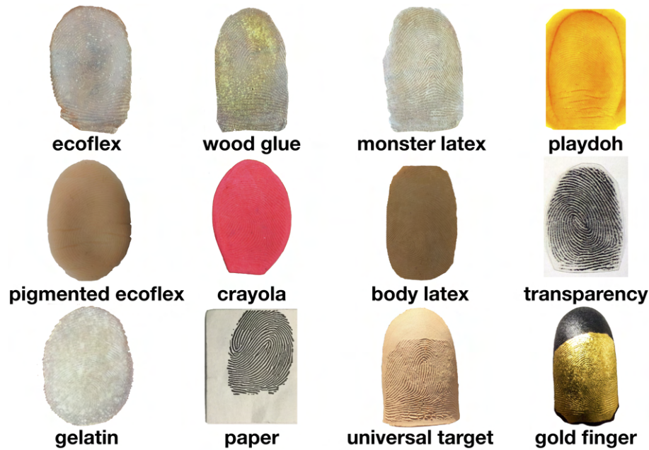
Figure 1.14 Examples of fingerprint spoofs made from different materials. The material variety demonstrates why it is difficult to develop a spoof detector which generalizes well across all material types.
