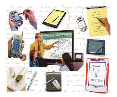
Figure 1.3: Devices that accept on-line handwritten data: From the top left, Pocket PC, CrossPad, Ink Link, Cell Phone, Smart Board, Tablet with display, Anoto pen, Wacom Tablet, Tablet PC.
