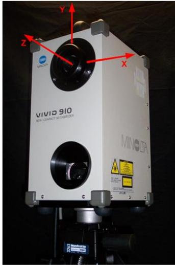
Figure 2.4: Scanner-based coordinate system.
