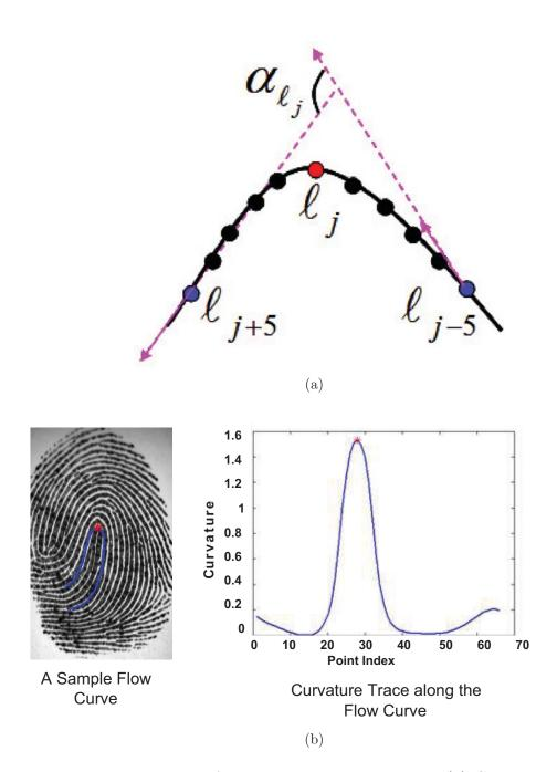
Figure 5.8: Determination of maximum curvature points. (a) Curvature estimation at point  $\ell_j$  and (b) trace of curvature for a sample flow curve along with the local maximum.
