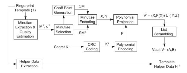
Figure 5.5: Proposed implementation of vault encoding.
