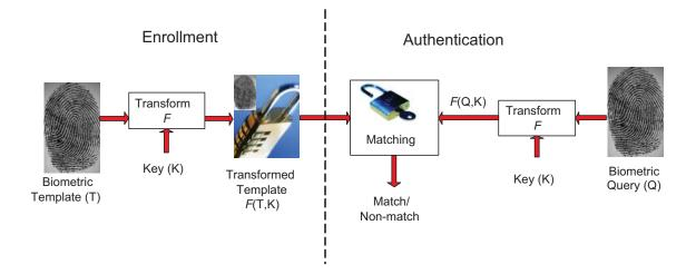
Figure 5.2: Authentication mechanism when the biometric template is protected using a feature transformation approach.
