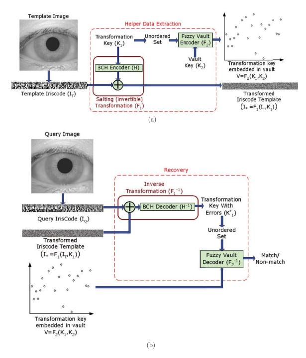
Figure 5.10: Schematic diagram of the iris cryptosystem based on iriscode features. (a) Enrollment or helper data extraction and (b) authentication or key recovery.
