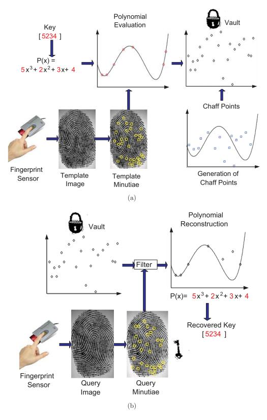
Figure 5.4: Schematic diagram of the fuzzy vault scheme proposed by Juels and Sudan [102] based on fingerprint minutiae. (a) Vault encoding and (b) vault decoding.
