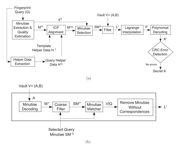
Figure 5.6: Proposed implementation of vault decoding. (a) Block diagram of the complete decoding process and (b) details of the filter used to eliminate the chaff points.
