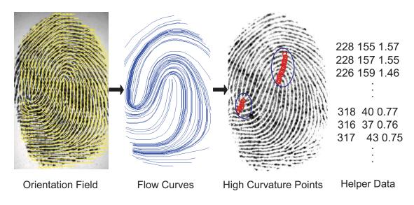
Figure 5.7: Algorithm for extraction of high curvature points.
