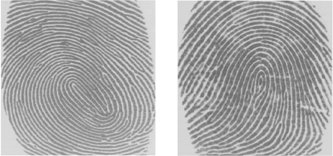
Figure 4.1: Examples of good quality live-scan fingerprint images, which were captured using a fingerprint scanner manufactured by Digital Biometrics.
