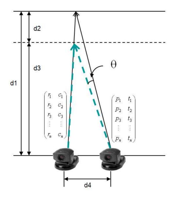
Figure 2.32. Calibration between static and PTZ cameras.
