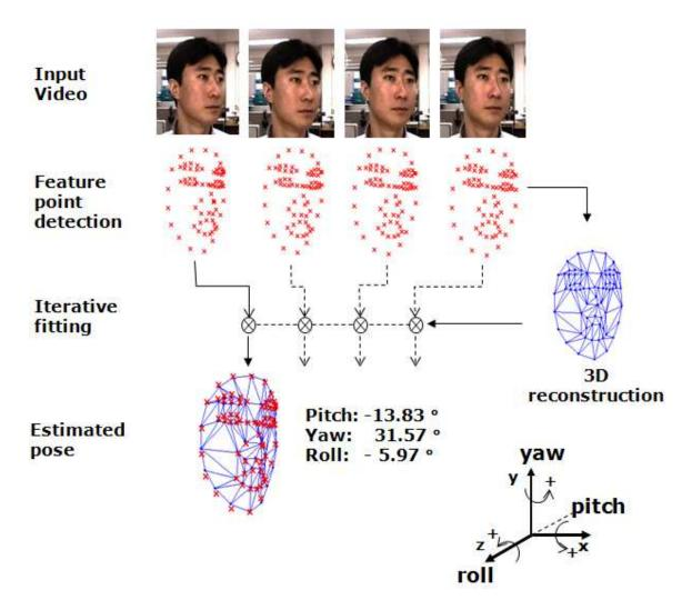
Figure 2.6. Pose estimation scheme.
