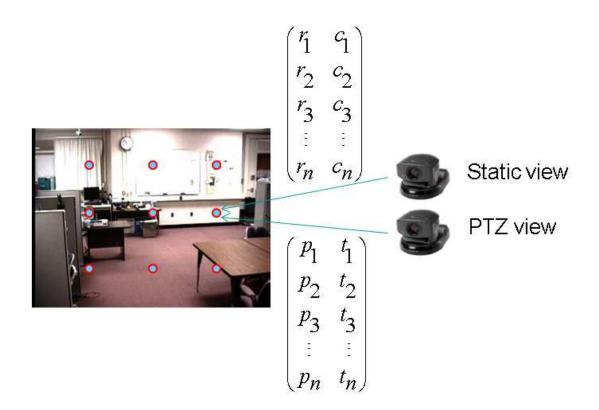
Figure 2.31. Schematic of camera calibration.
