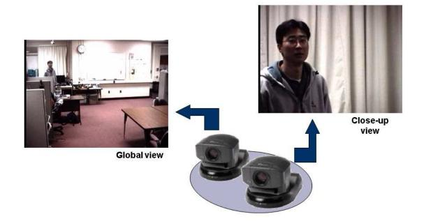
Figure 2.30. Schematic of face image capture system at a distance.
