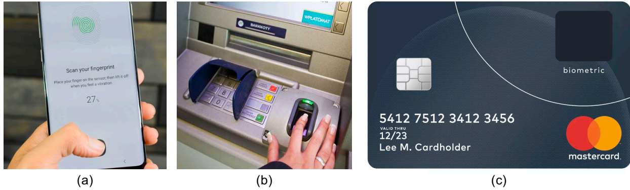
Figure 1.8 Fingerprint-based authentication is used in many commercial applications, including executing financial transactions, unlocking devices, access control, etc. (a) A user enrolling their fingerprint in Samsung Galaxy S10 with an in-display ultrasound-based fingerprint sensor, (b) user authentication in ATM transactions, and (c) biometric-enabled payment cards with embedded fingerprint sensor and on-card storage for fingerprint template.
