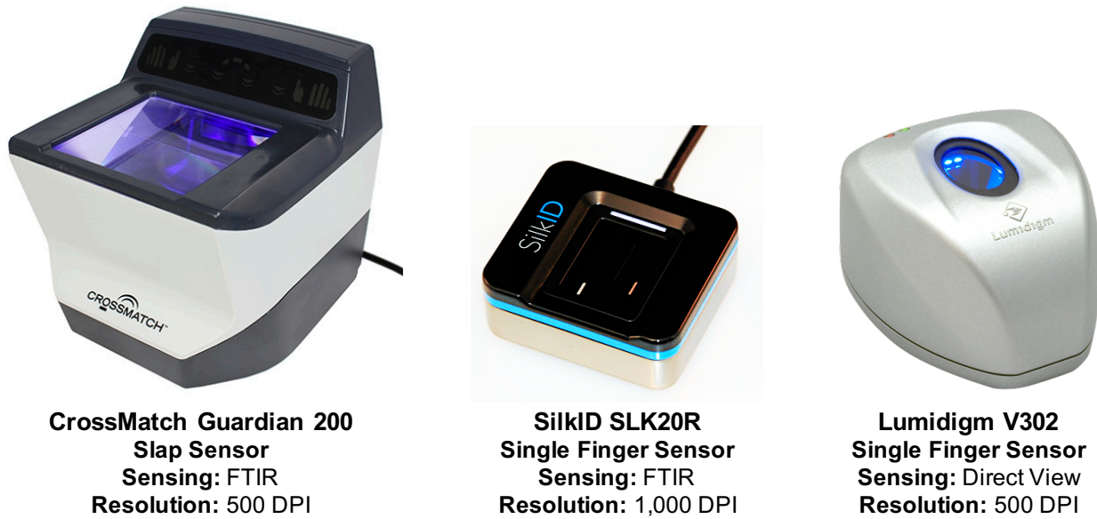
Figure 1.14 Optical fingerprint sensors utilized in our experiments.
