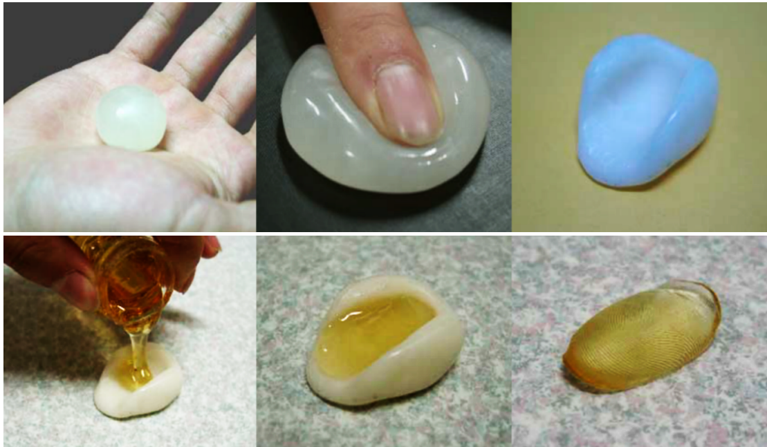
Figure 1.19 Example procedure to create an artificial fingerprint directly from a live finger. Plastic is used to create the mold and gelatin is used as the casting material. Image reproduced from [105].
