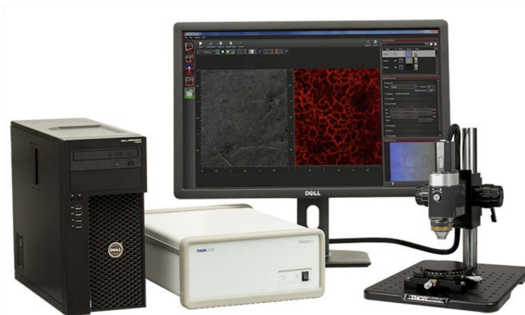
Figure 4.7 Setup of a THORLabs Telesto series Spectral-domain OCT scanner (TEL1325LV2). Image taken from [154].
