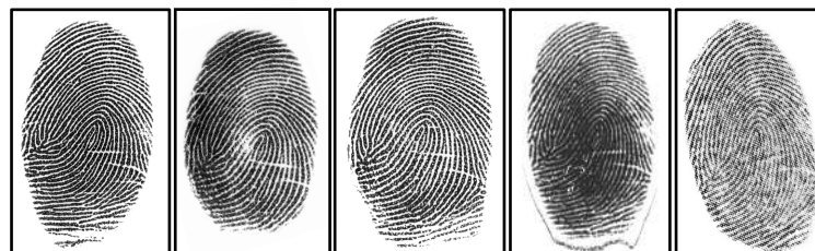
Live Fingerprint PlayDoh (Orange) Silicone (Ecoflex) 2D Printed (Transparency Film) 2D Printed (Matte Paper)
