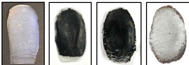
Ecoflex (Silicone) Ecoflex with Nanotips Coating Ecoflex with BarePaint Coating Ecoflex with Silver Colloidal Ink Coating
