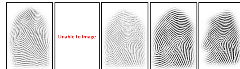
Live Fingerprint PlayDoh (Orange) Silicone (Ecoflex) 2D Printed (Transparency Film) 2D Printed (Matte Paper)
