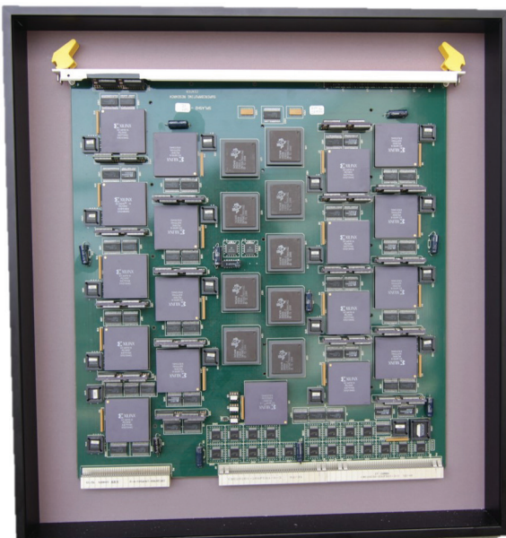
Figure 1. The Splash 2 board consisting of an array of Xilinx 4010 field-programmable gate arrays. A sequential point-matching algorithm (assuming an average of 65 minutia points per fingerprint) executed on a Sun SPARC-station 20 runs at 100 matches per second. The same algorithm implemented on Splash 2 running at 1 MHz executes at 6,300 matches per second. (Source: Duncan Buell, University of South Carolina.)
